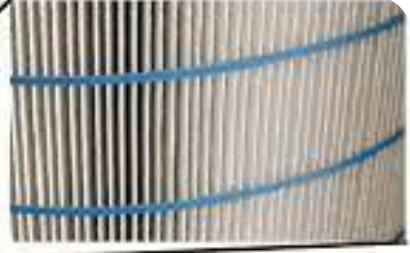
View of Pleats in Cartridge Filter
